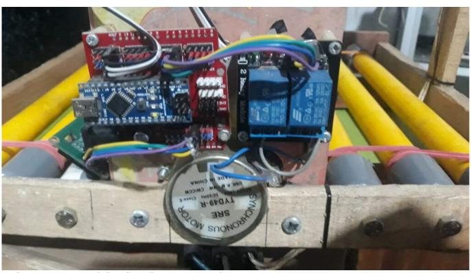
Arduino Nano, Modul Relay, dan Motor Sinkron
